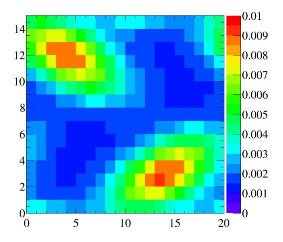
It reflects relatively frequent case of *kinematic reweighting* using the transverse momentum and rapidity. Typically one has enough events to make fine-binned one-dimensional reference distributions, but two-dimensional distributions can be obtained only with relatively coarse binning scheme.
